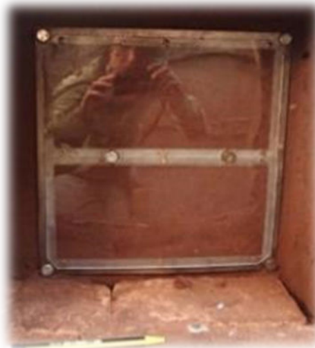
Root windows to monitor root dynamics and functioning
